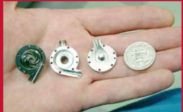
Inside view of Pediaflow pump for heart assist that is barely the size of a U.S. quarter.
