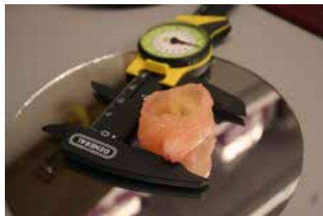
A clinically-sized human trileaflet heart valve made in the Butcher Lab using 3D printing of biological hydrogel polymers.
